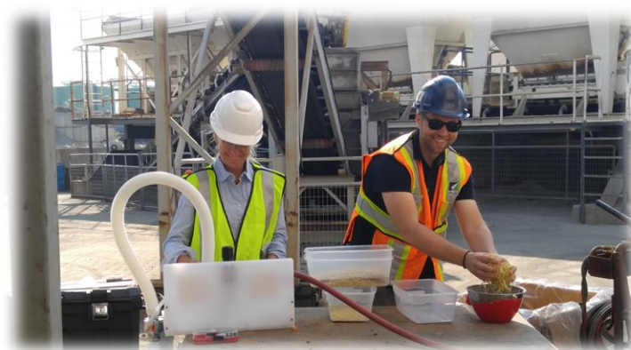
The Line-Vac® is used to transport ACE Fiber™ to the RAP Collar at a Drum Plant
