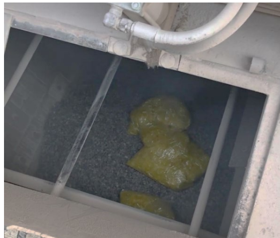
Figure 4: Manual Bag Feed at Batch Plant.
