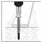
3. Using an impact or manual wrench, insert anchor into hole and tighten anchor until fully seated.
