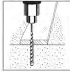
1. Using a carbide drill bit, drill a hole at least 1/4" deeper than anchor embedment.
