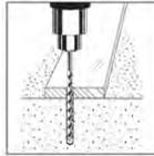
1. Using a carbide drill bit, drill a hole at least 1/4" deeper than anchor embedment.
